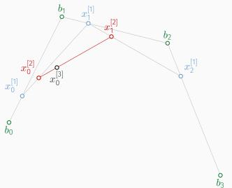
Repeat for the last segment to obtain  $\beta_3(\frac{1}{4};b_0,b_1,b_2,b_3)=x_0^{[3]}$ .
