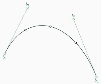
Complete curve  $\beta_3(t; b_0, b_1, b_2, b_3)$ .
